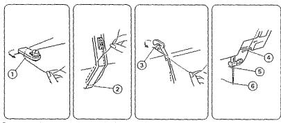
Raise take-up lever to its highest position by turning hand wheel toward you. Raise presser foot lever.
